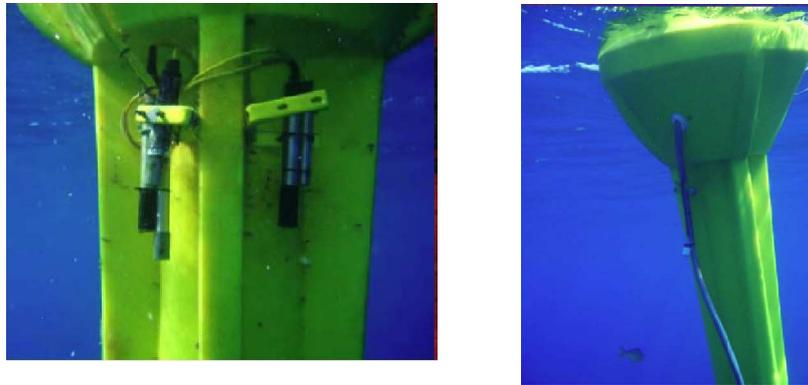
Figure 4: Sensor arrangement: classical buoy (above), Hidroboya (below).
