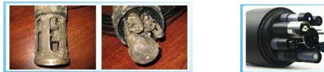
Figure 5: Sensors affected by fouling (above). Hidroboya keeps sensors clean (below).
