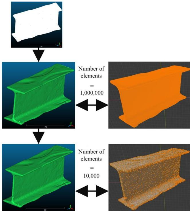
Figure 4. Reduction of the number of elements in the model to achieve the minimum rendering size that provides a final model for proper calculation.
