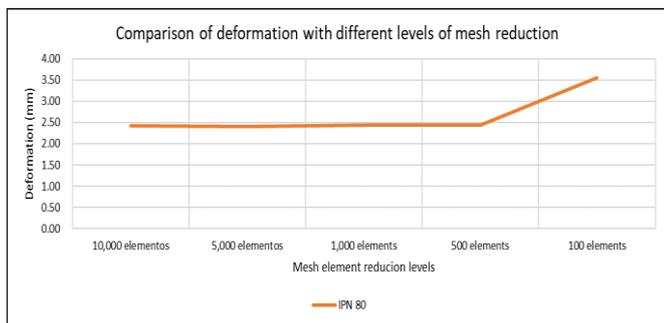
Figure 5. Deformation graph at beam end according to number of rendering elements.
