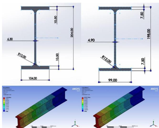
Figure 7. Calculation of an IPE 200 with the possible maximum and minimum measurements according to the standards due to its manufacturing process.
