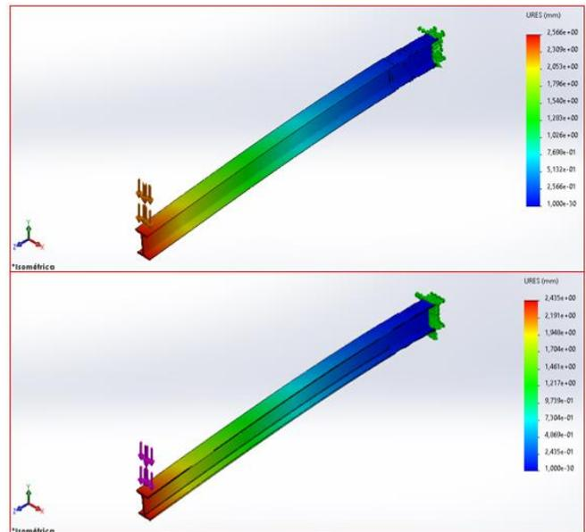
Figure 3. Calculation of the beam by extruded slices and rendering.
