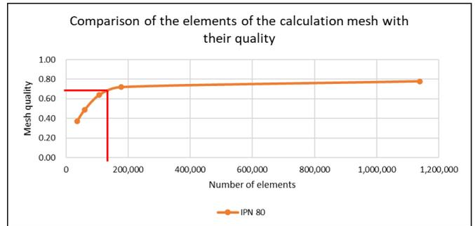
Figure 6. Quality of the mesh depending on the number of elements in the mesh.
