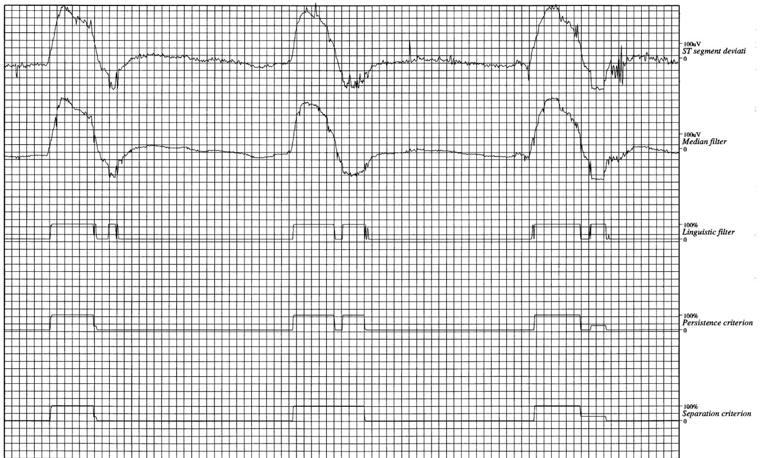
Fig. 5. Example of the transformation of the trend diagram of an ST segment amplitude by the application of the successive stages of our ischemic episode detection algorithm (five squares are equivalent to 1 min). It can be appreciated that the patient suffers several ST episodes (extracted from recording eO113 of the European ST-T Database).
