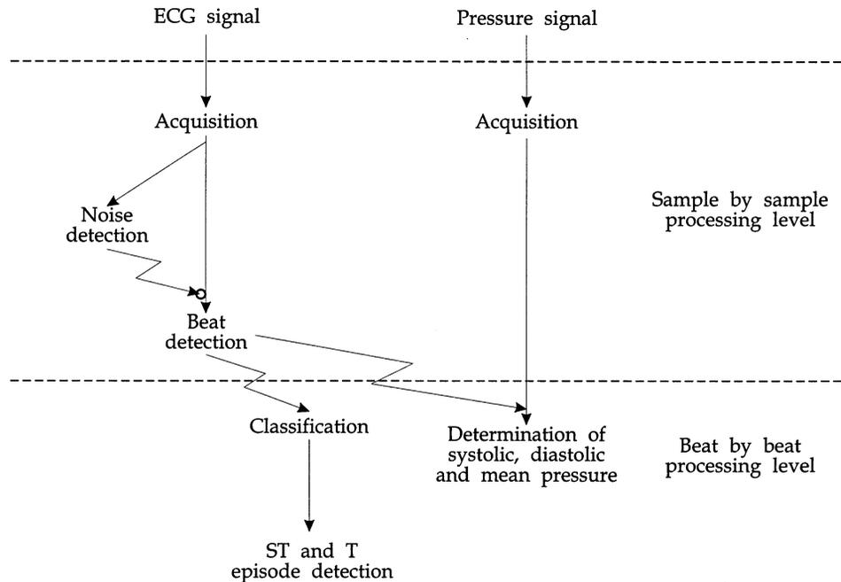
Fig. 2. Structure of SUTIL at the processing block level (the dashed arrows indicate situations where new routines are triggered,  $\rightsquigarrow$ ; or disabled,  $-o$ ).
