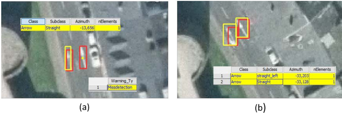
Figure 9. The GIS layer obtained with the proposed algorithm (yellow bounding boxes) can be visualized over an ortophoto, and compared with respect to a ground truth or data from a previous survey (red bounding boxes). (a) Misdetctions due to occlusions or algorithm failures are automatically found in order to assist the maintenance process.
