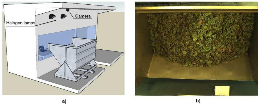
Fig. 1. Image acquisition system: a) Diagram of the grape reception point; b) Obtained image of the container surface
