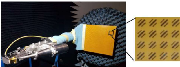
Fig. 7 Picture of the prototype in the anechoic chamber and detail of the printed dipoles.
